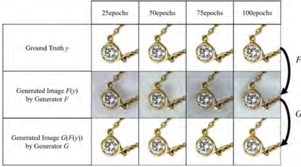
Fig. 3 The generated image F(y) from the ground truth image y and the generated image G(F(y)) by the generator G in the learning process of CycleGAN
